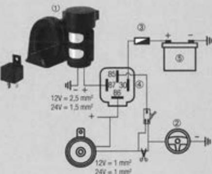
Wiring diagram for cars with ground lead to horn button.
